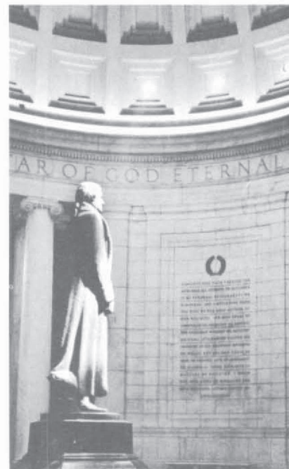
SEARCHLIGHTS are mounted 8 ft apart behind rotunda ceiling, approximately 50 ft above floor, and aimed through oval-shaped openings cut in the Georgia marble ceiling. Average intensity on statue's surface from 12 500-watt units is 200 footcandles.
