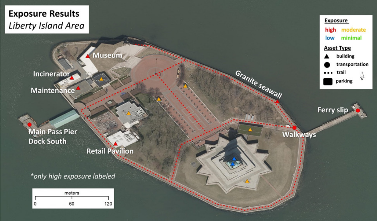
Figure 1. STLI exposure results summary for the Liberty Island Area. Only high exposure assets are labeled. Background map is ESRI streaming imagery.
