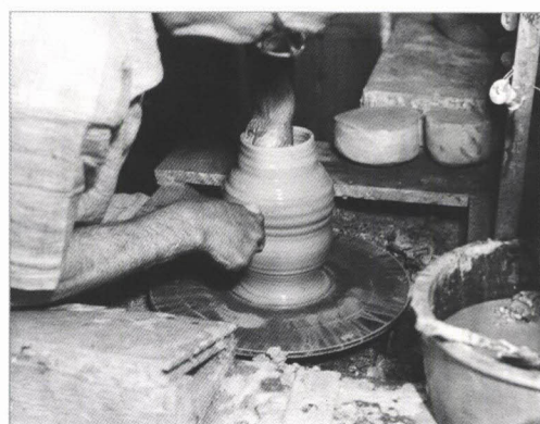
13 THROWING: A knuckle draft for shaping and filling out. The tips of the inside fingers are just below the knuckles as usual, pressing out but gently.
