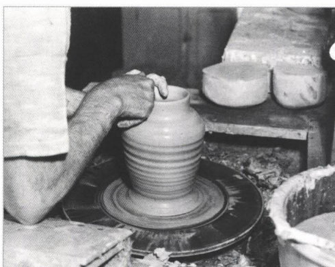
12 THROWING: Drawing in the top with the trueing hold. As the rim is trued it is pushed towards the center to the desired diameter.
