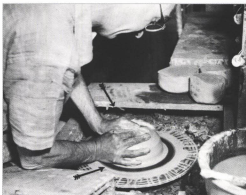
5 THROWING: Centering the ball. Arrows show directions of force, which must be applied strongly.
