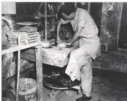
6 THROWING: Opening the ball with the thumb of one hand and fingers of the other. The wheel is an old treadle model built into the corner of the shop. Note the waterbowl, the upright for the throwing gauge, and, to the left, the scaler for weighing out balls, the wedging block, and the plate lifters on the stack of slat batts.
