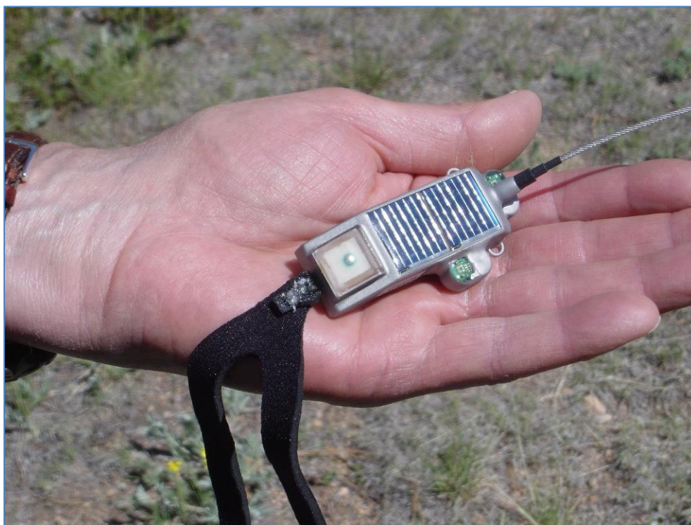
Figure 1. Solar powered satellite tracking unit with harness deployed on ospreys from Rocky Mountain NP. Two geolocators are visible on right side on bottom just left of loop and under the base of the antennae.
