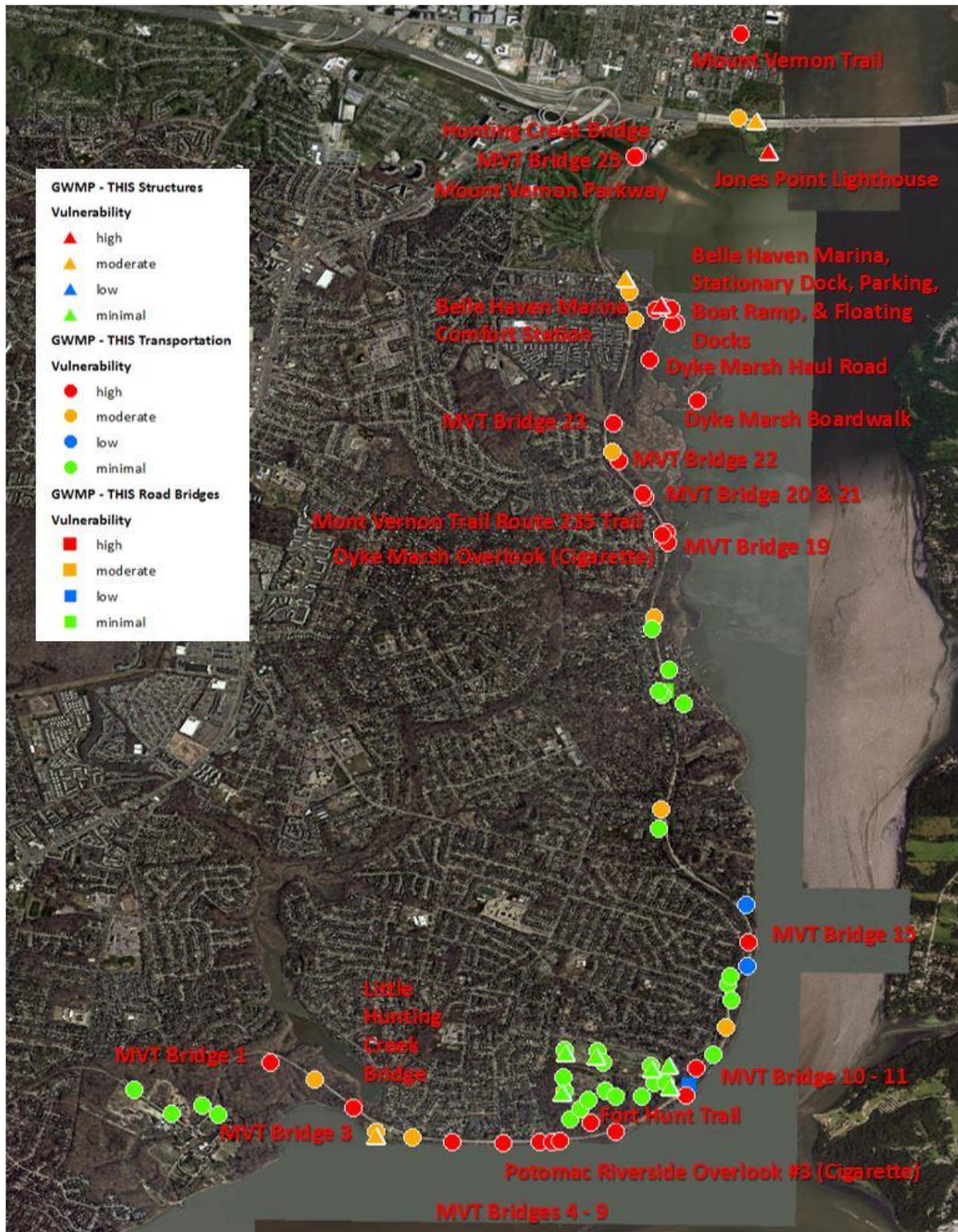
Figure 5. Mapped vulnerability results for the southern GWMP assets (from Alexandria south to Mount Vernon). Only the high vulnerability assets are labeled. Background is aerial imagery from the ESRI streaming layer (see Digital Data Sources).
