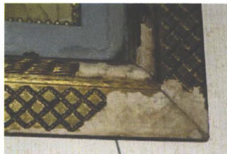
Insect-damaged molded decorative papier mache surface
