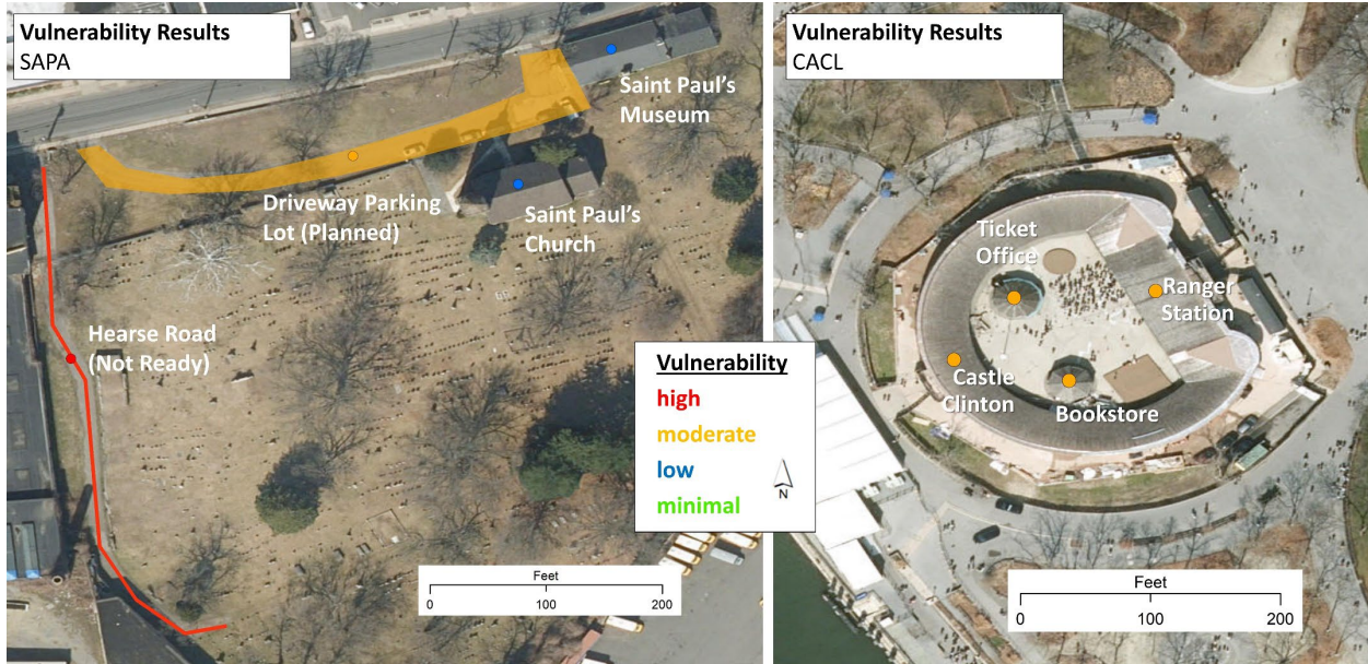
Figure 3. Vulnerability results for SAPA (left) and CACL (right). Parking lots are represented by polygons and roads by lines. Only high exposure assets are labeled. Background map is ESRI streaming imagery.
