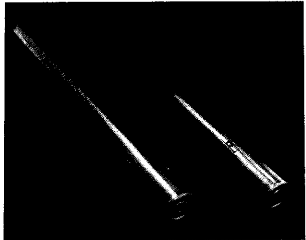
Left, a normal uranium fuel rod, manufactured using the coextrusion process, ready for insertion into N Reactor. Right, an N Reactor fuel element holding a lithium aluminate target used for making the "coproduct" (tritium), in the late 1960s.
