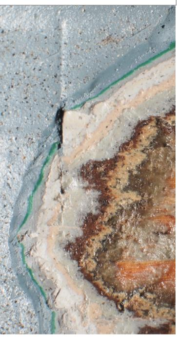
Micrograph of finishes applied to 493-3 east clapboards.
