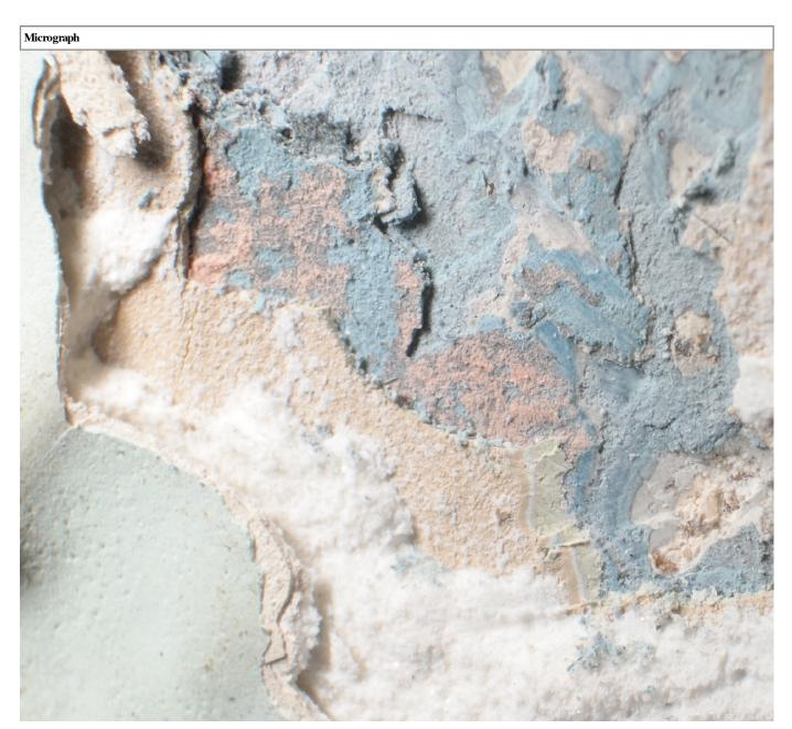
Micrograph of finishes applied to 493-2 interior east room wall plaster.
