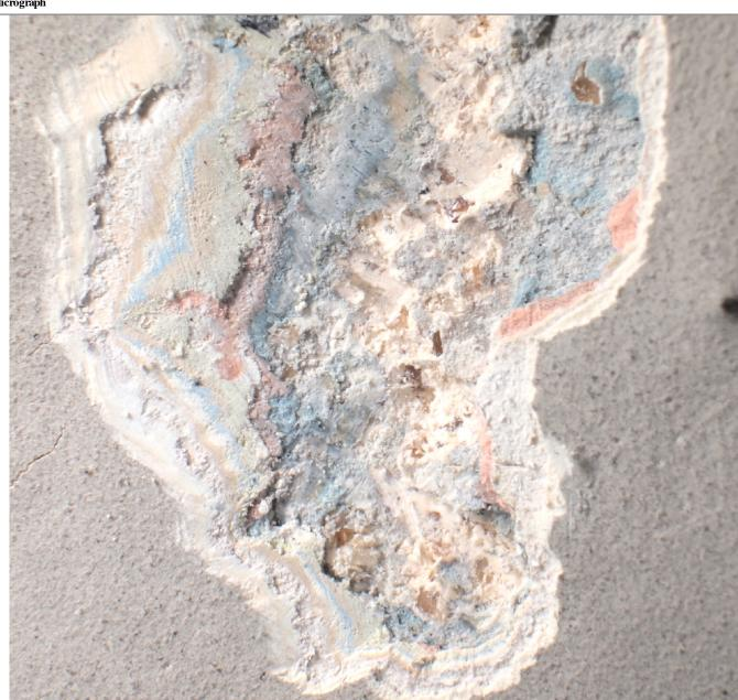
Micrograph of finishes applied to 493-2 interior east room ceiling plaster.
