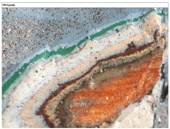
Micrograph of finishes applied to 493-3 east clapboards.
