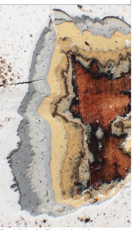
Micrograph of finishes applied to 493-1 east window, lower sash stile.
