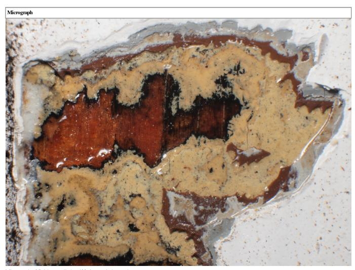
Micrograph of finishes applied to 493-6 east window sash.
