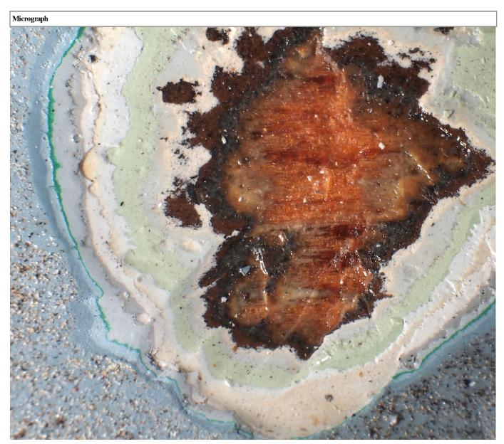
Micrograph of finishes applied to 493-6 east clapboards.
