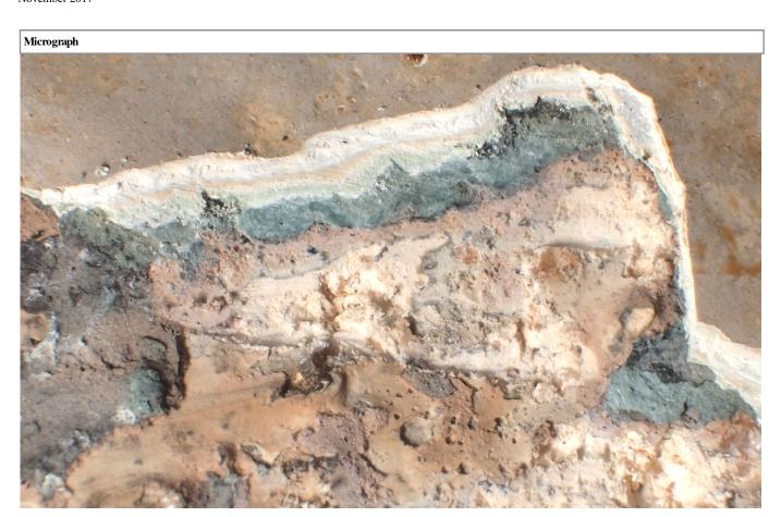
Micrograph of finishes applied to 493-2 interior west room ceiling plaster.
