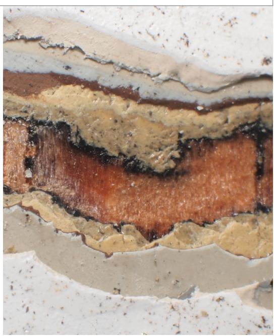
Micrograph of finishes applied to 493-3 east window sash.
