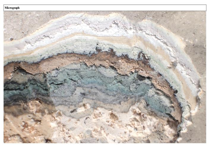
Micrograph of finishes applied to 493-2 interior west room wall plaster.
