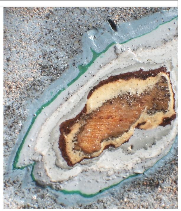
Micrograph of finishes applied to 493-1 east clapboards.
