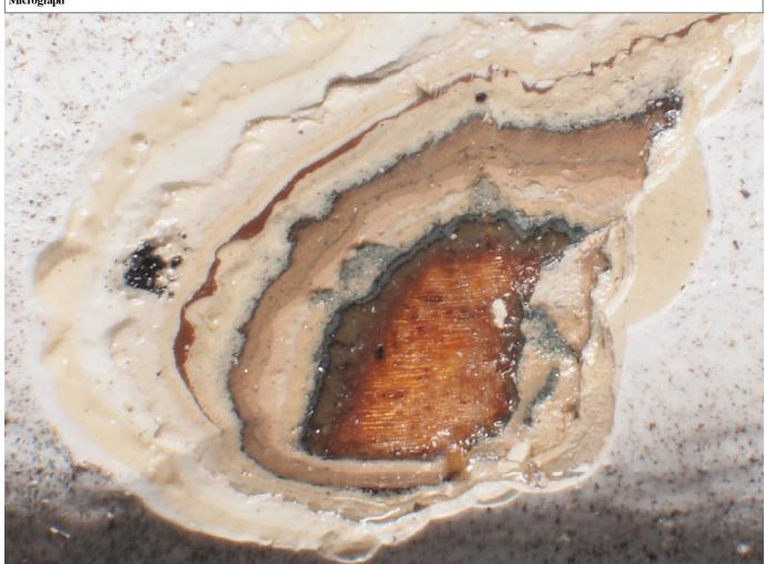
Micrograph of finishes applied to 493-2 east door rail.
