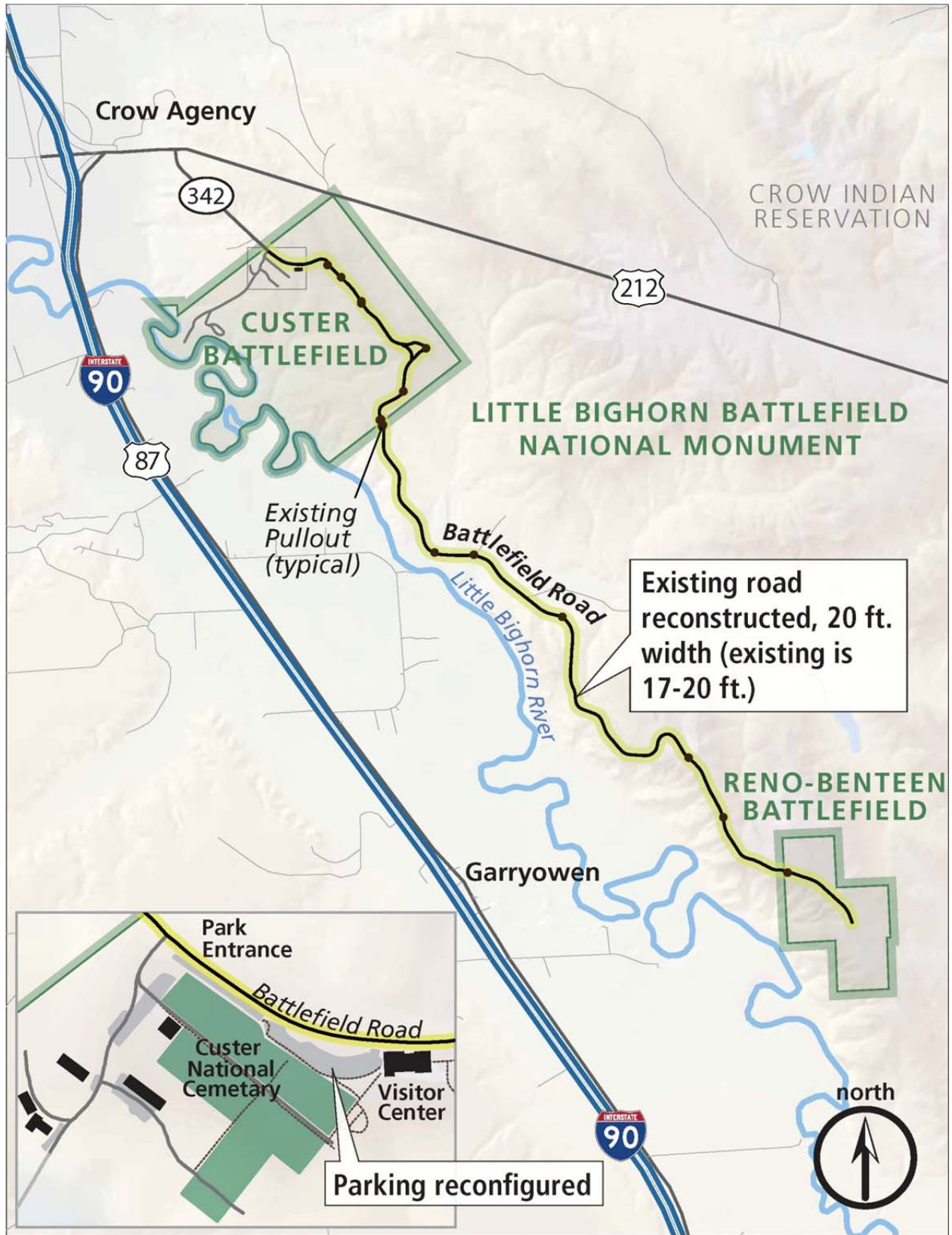
Figure 5. Option I: Repair Existing Road
