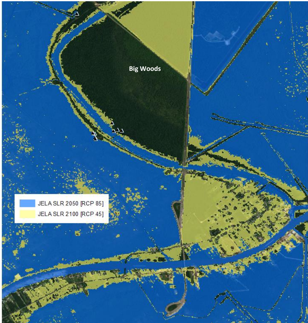
Figure 8. Map showing the difference in coverage between the 2050 SLR model scenario (8.5 RCP) and the 2100 SLR model scenario (4.5 RCP) within the Barataria area of JELA. The yellow represents the additional area that is covered by the 2100 SLR model that is not covered by the 2050 model. These areas represent inundation of the ground surface and do not represent water height. Areas without blue or yellow are represented by aerial imagery.
