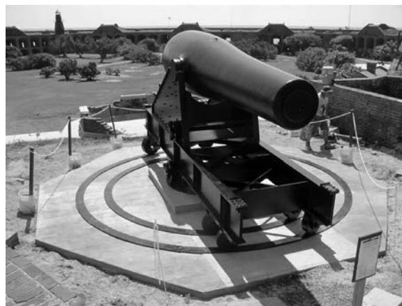
Figure 27. Conserved Rodman cannon mounted on reproduction iron carriage and gun platform, 2011. (NPS image)
