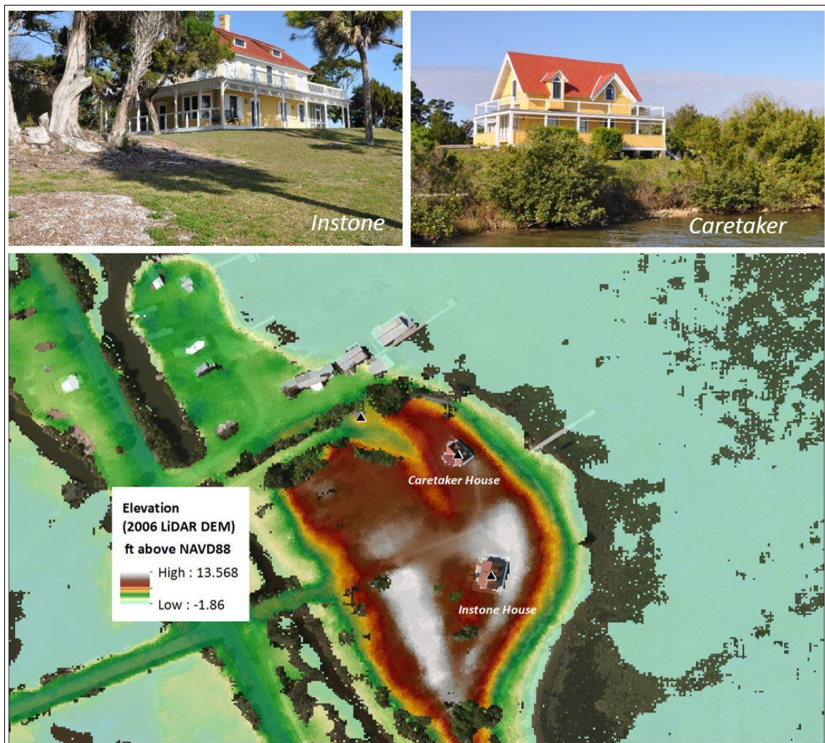
Figure 5. Historic structures within the Seminole Rest district of the park. Top: Photos of the Instone and Caretaker Houses. Bottom: LiDAR DEM for this area of the park. Notice the dark brown and white shading near the two historic houses, representing higher elevations (between 10 and 13 feet above NADV88). These structures were built upon an artificial shell mound.
