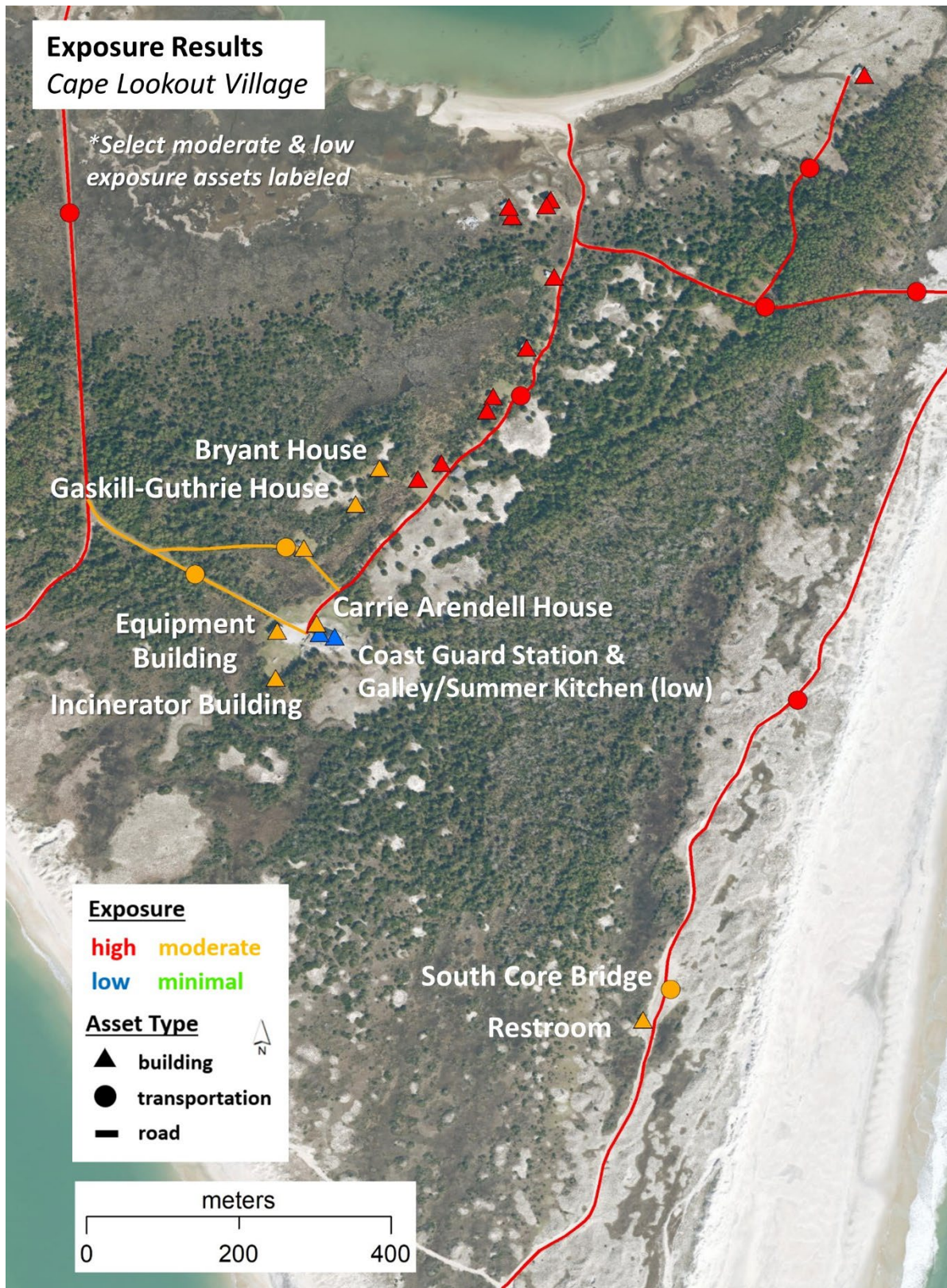
Figure 5. Exposure results for the Cape Lookout Village area of CALO. Select moderate and low exposure assets are labeled. Background is ESRI streaming imagery.
