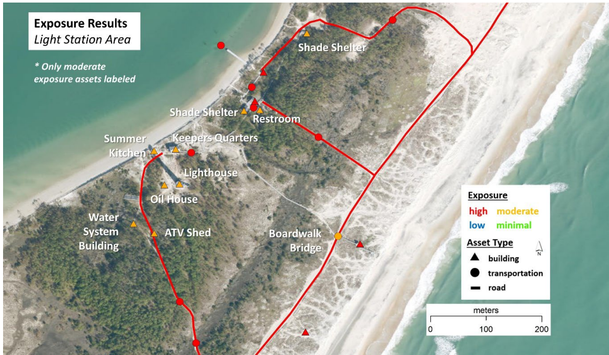
Figure 2. Exposure results for the Light Station area of CALO. Only moderate exposure assets are labeled. Background is ESRI streaming imagery.
