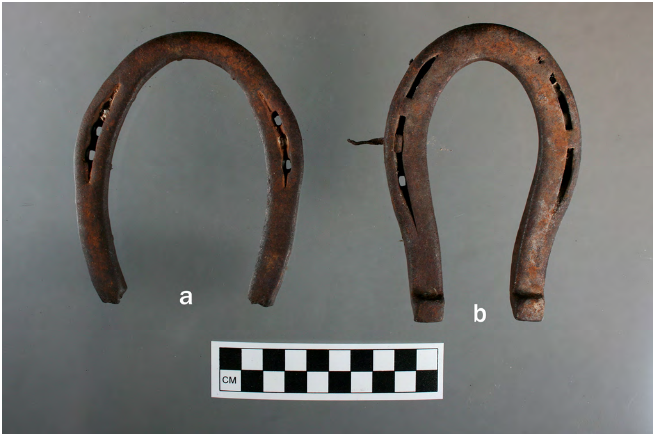
Figure 6-III.115 Horseshoe and muleshoe: (a) Handmade 6-hole hind shoe; (b) Machine-made 8-hole muleshoe.
