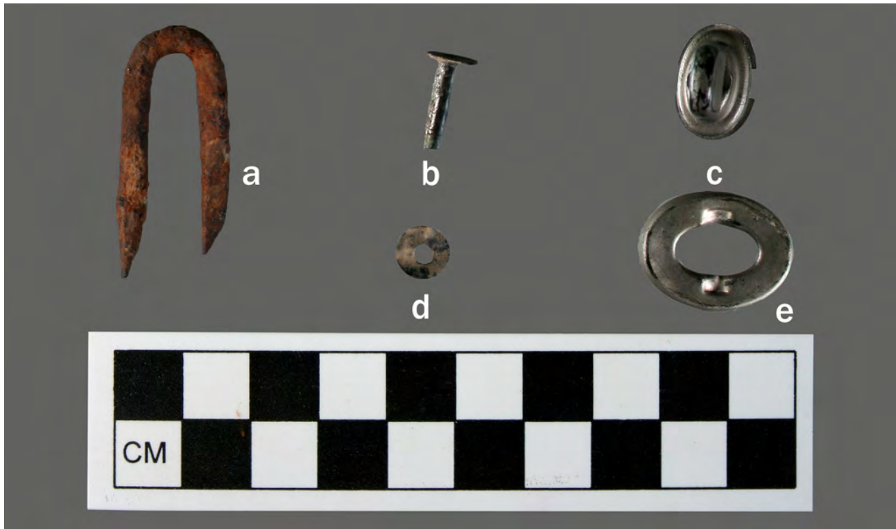
Figure 6-III.104 Various fasteners: (a) Fencing staple; (b) Rivet; (c) Twist-lock fastener; (d) Rivet washer; (e) Twist-lock fastener receptacle.
