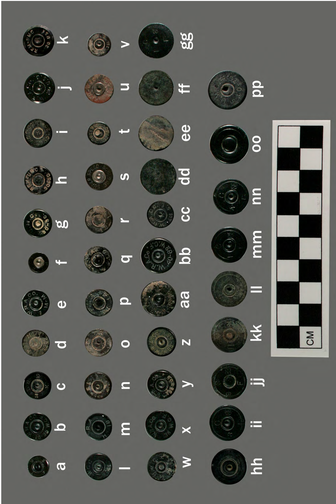
Figure 6-III.130 Rifle cartridge casings: (a) 5.56x45mm; (b) .25-35; (c-e) 7mm Mauser; (f) .30 Carbine; (g-i) .30-30; (j-k) .30-40 Krag; (l-s) .30-06; (t) .32-20; (u) .32-40 Remington; (v) .351 Winchester; (w) .38-40 Winchester; (x-z) .38-55; (aa) .38-56; (bb) .40-82 Winchester; (cc) .401; (dd) .41 Swiss; (ee-gg) .45-70 Benét primed; (bb-nn) .45-70 Externally primed; (oo) .50-45 Cadet; (pp) .50-70.
