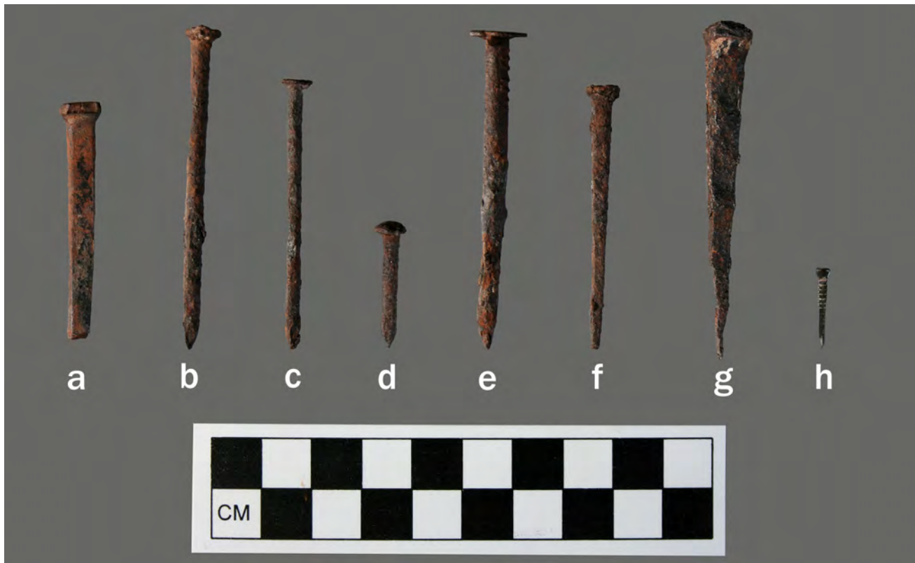
Figure 6-III.103 Nails: (a) Cut nail, 6d; (b) Wire nail, 8d; (c) Wire nail, 6d; (d) Wire nail, domed head, 2d; (e) Wire nail, large head, 8d; (f) Boat nail, 6d; (g) Wrought nail, 8d; (h) Brass soling nail.
